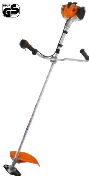
**24.1 cm<sup>3</sup>, 0.9 kW/1.2 hp, 4.9 kg<sup>①</sup>.** Lightest brushcutter in this segment. STIHL 1-point anti-vibration system, STIHL Easy2Start, bike handle, engine controls with ECOSPEED partial load function, 2-MIX engine, straight shaft, double shoulder harness.
