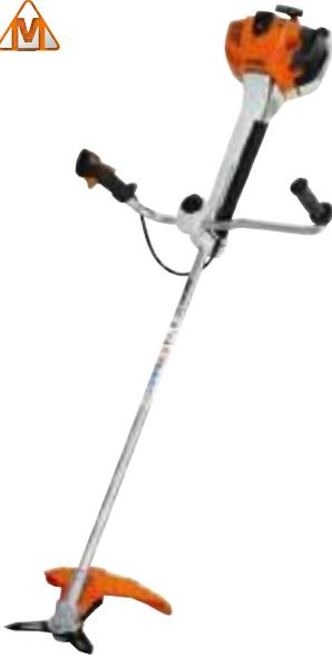
**37.7 cm<sup>3</sup>, 1.7 kW/2.3 hp, 8.5 kg<sup>Ⓞ</sup>**. For mowing tough grass. STIHL 4-point anti-vibration system, STIHL Easy2Start, multi-function handle, bike handle, tool-free handle adjustment, 2-MIX, STIHL M-Tronic engine with ADVANCE PLUS universal harness.
