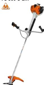
**37.7 cm³, 1.7 kW**/2.3 hp, **8.5 kg** <sup>©</sup>. For mowing tough grass. STIHL 4-point antivibration system, STIHL Easy2Start, multi-function handle, bike handle, tool-free handle adjustment, 2-MIX, STIHL M-Tronic engine with ADVANCE PLUS universal harness.
