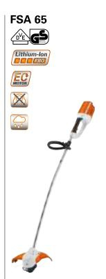
Battery brushcutter for thinning work. Cutting circle diameter of 300 mm, soft grip, infinitely variable loop handle, the mowing line automatically readjusts when the mowing head is tapped on the ground. Weight: 2.7 kg<sup>©</sup>.
