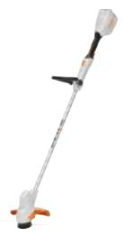
Lightweight battery brushcutter with high mowing performance. Cutting circle diameter of 280 mm, adjustable shaft length at the press of a button and handle adjustment without any tools required, and soft handle with control lever. The mowing line automatically readjusts when the mowing head is tapped on the ground. Weight: 2.5 kg<sup>2</sup>.
