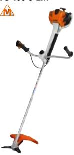
**45.6 cm³, 2.2 kW**/3.0 hp, **8.5 kg**<sup>©</sup>. For working in challenging areas of tough grass. STIHL 4-point anti-vibration system, STIHL Easy2Start, multifunction handle, bike handle, tool-free handle adjustment, 2-MIX engine, STIHL M-Tronic, with ADVANCE PLUS universal harness.
