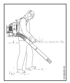
Place the unit securely on the ground and make sure that bystanders and loose objects are well clear of the nozzle outlet
