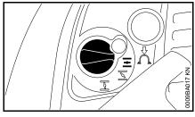
Choke knob automatically returns to the run position when the throttle trigger is operated.
