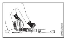
Place the unit securely on the ground and make sure that bystanders and loose objects are well clear of the nozzle outlet.
