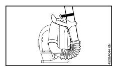
Secure the blower tube to the handle on the backplate with the hook and loop fastener.
