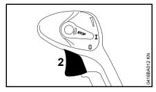
• Operate the throttle trigger (2).
