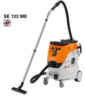
**1.4 kW, 250 mbar, 4,500 l/min.** Full wet and dry vacuum cleaner with automatic switch-on function when used in conjunction with electric tools. Dust class M with automaticfilter cleaning without loss of suction power, automatic volume flow monitoring, infinitely variable speed control, with adapter plates for carrying tool boxes, anti-static accessories also for extraction on battery-powered electric power tools.
