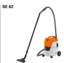
**1.4 kW, 210 mbar, 3,600 l/min.** For getting rid of dust, dirt and liquids indoors and outdoors. Wet and dry vacuuming options, blower function by moving the suction tube to the exhaust port, multiple filter system, filter cleaning, switchable floor nozzle, universal nozzle, crevice nozzle.
