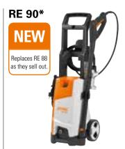
10-100 bar, 520 l/h, 9.6 kg. Lightweight and compact 100 bar high-pressure cleaner with basic features. Aluminium pump head, integrated wheel kit, cleaning agent spray set with spray bottle, rotary nozzle, adjustable fan jet nozzle with pressure regulation, anti-drill, quickrelease coupling on the lance, park position for switching off the sprayer during breaks in work, 6 m high-pressure hose, transport handle.
