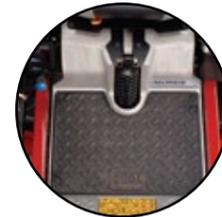
**The Suspension System** controls the motion of the operator platform, providing a smoother ride than a standard suspension seat.
