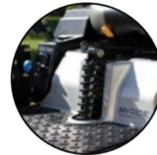
**Three Coil-Over-Shock Absorber Assemblies** suspend the operator platform for cushioning you'll appreciate in your feet, knees and back — all without sacrificing quality of cut like other suspension systems.
